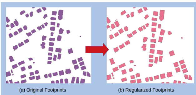
Fig. 4. Buildings' footprint polygonization and regularization process: (a) model original output masks are first transformed into polygons and then (b) regularized to achieve buildings-like shape.
