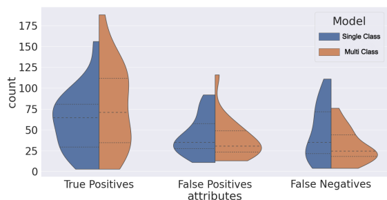
Fig. 3: Violin Plots showing different metrics probability density distributions to compare the instance segmentation performance between the single and multi-class models.
